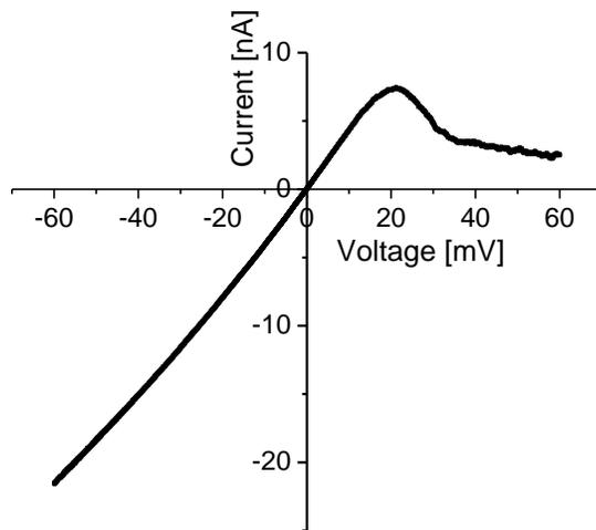
**Figure 6** The strongly non-linear I-V curve recorded for a population of lysenin channels inserted into an Asolectin-based bilayer membrane indicated that positive voltages greater than  $\sim 20\text{mV}$  induced channels' closure, and that the lysenin channels were directionally inserted.
