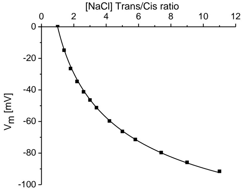
**Figure 11** The use of neutral lipids preserved the ionic selectivity of the lysenin channels and indicated a permeability ratio of  $18.39 \pm 0.38$  for cations over anions. The almost identical behavior of charged and neutral lipids suggests that the selectivity filter is part of the lysenin channel's structure.
