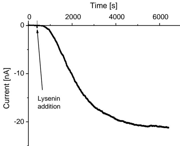
**Figure 5** Addition of lysenin to the *trans* reservoir under voltage clamp conditions ( $V = -60\text{mV}$ ) yielded an ionic current indicative of channel insertion. The macroscopic current stabilized after  $\sim 2$  hours indicating the completion of the insertion process.
