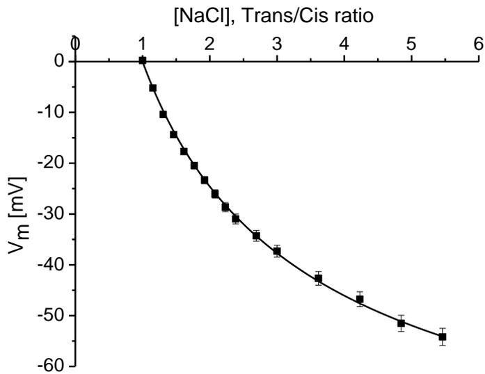
**Figure 8** NaCl addition to the *trans* side elicited the development of transmembrane voltages (symbols) matching the GHK equation (full line) for a permeability ratio of  $18.3 \pm 1.34$  ( $n=3$ ) for cations over anions.
