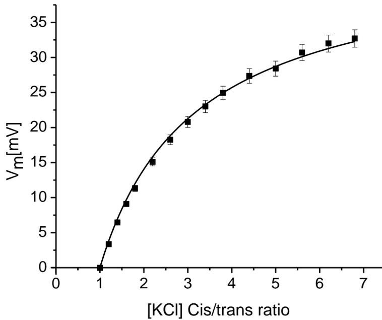
**Figure 9** KCl addition to the *cis* side elicited the development of transmembrane voltages (symbols) matching the GHK equation (full line) for a permeability ratio of  $2.55 \pm 0.34$  ( $n=3$ ) for cations over anions.
