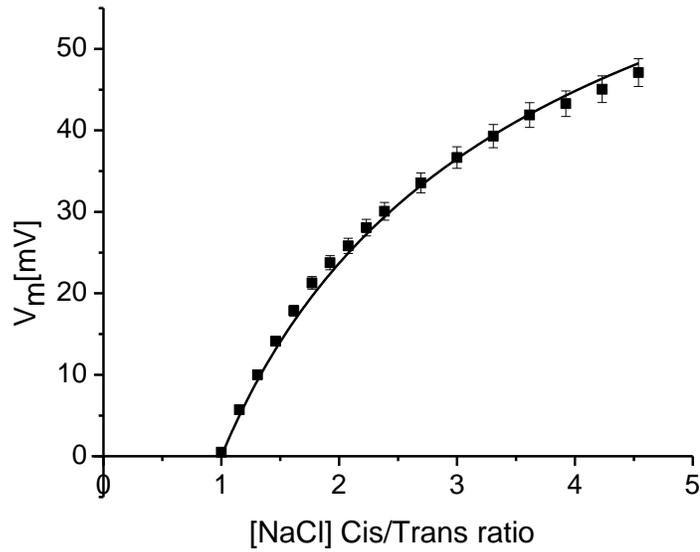
**Figure 7** Addition of NaCl to the *cis* side elicited the development of transmembrane voltages (symbols) matching the GHK equation (full line) for a permeability ratio of  $6.38 \pm 0.16$  ( $n=3$ ) for cations over anions.
