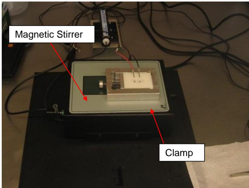
**Figure 2** Picture of the BLM Chamber setup in addition to the magnetic stirrers and clamp
