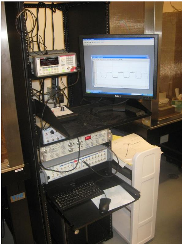
**Figure 4** Recording Setup (Axopatch 200B Amplifier, DigiData 1440 Digitizer)
