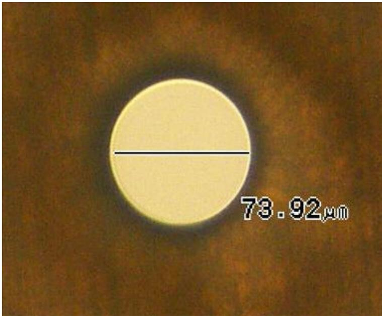
**Figure 3** Microscope Picture of Teflon Film with Hole
