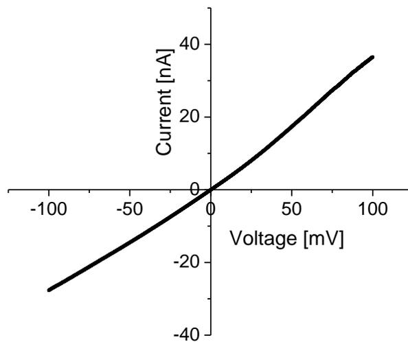
**Figure 10** The linear I-V curve recorded when working with neutral lipids shows no abrupt drop in the macroscopic current and indicates the absence of a voltage gating mechanism in play.
