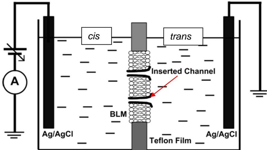
**Figure 1** BLM Chamber Setup: PTFE® reservoirs setup
